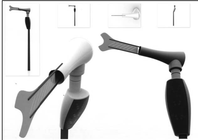
Figure 2. The perspective views of the proposed windsock.
