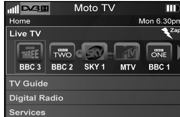
Figure 1. The “Zap to” concept featuring dynamic manipulation of the channel order based on the currently screened content’s match to the user’s learnt preferences.
